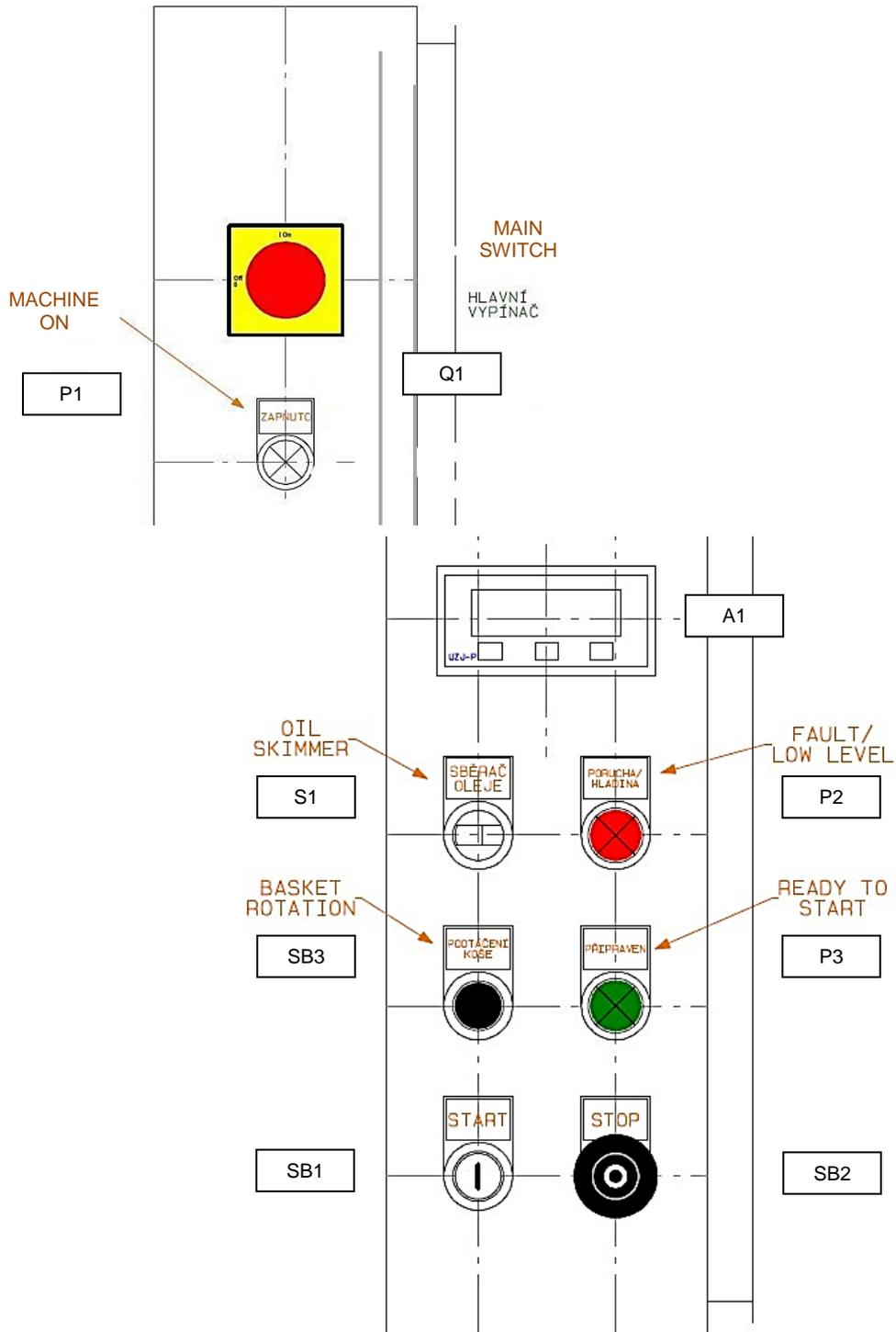
Fig. 7 shows the control panel of the electric switchboard
