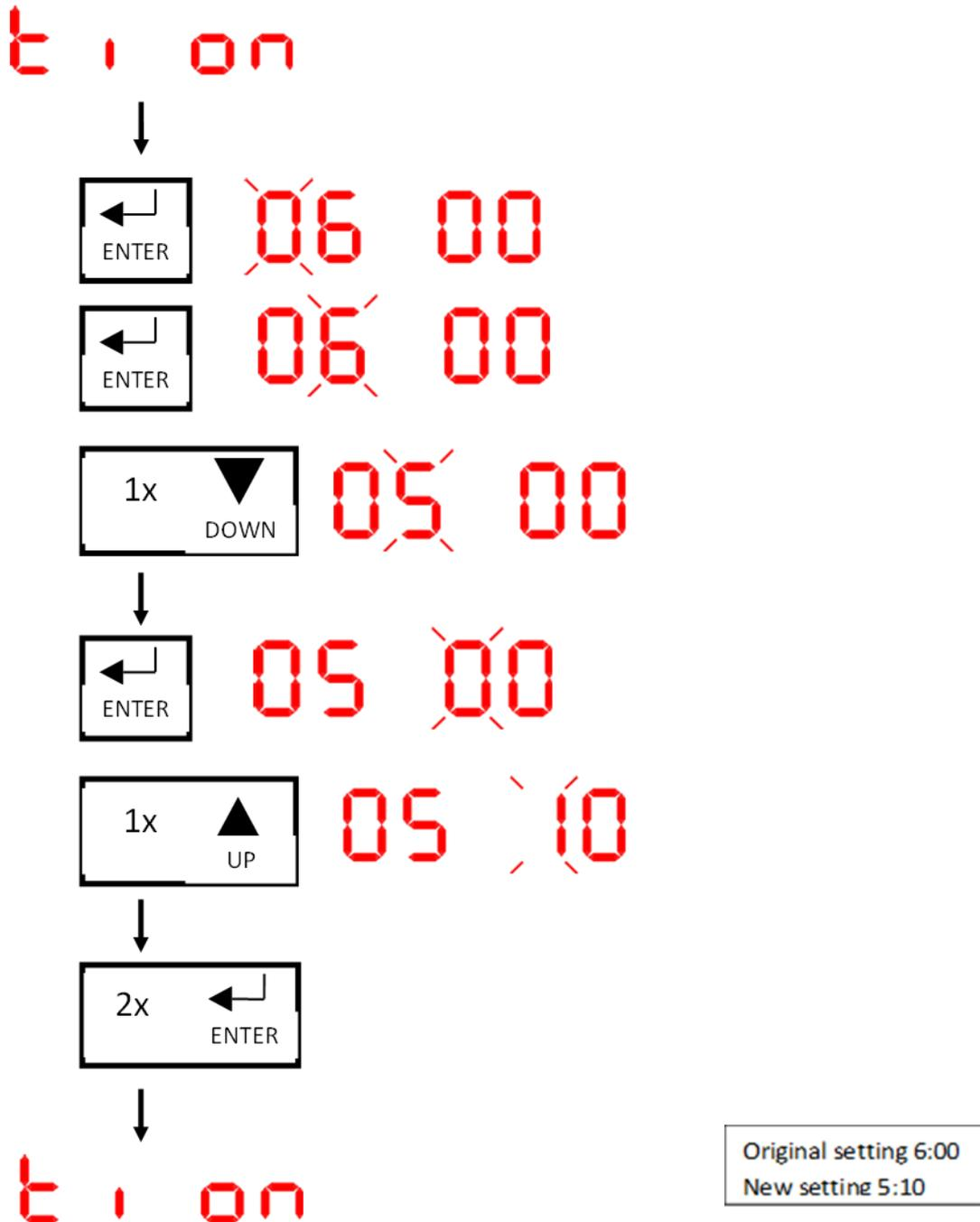
Figure 6.3.2-7 Illustration of the procedure for changing the parameters of switching the heating time on and off
