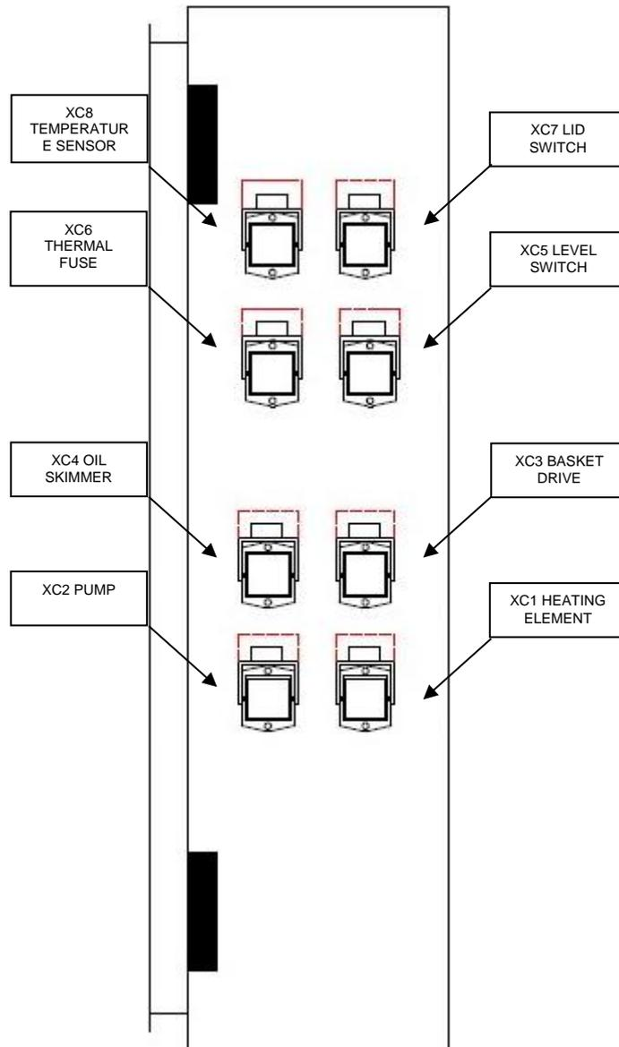
Fig. 7a shows the connectors for connection of electric units and sensors of the machine
