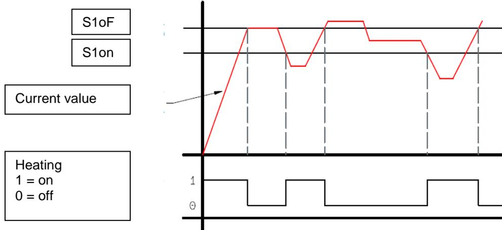
Figure 6.3.2-4 Illustration of heating element switching
