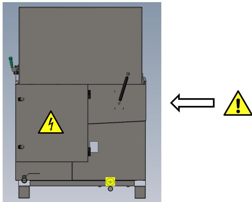
Fig. 6.2 Layout of warning symbols on the rear and right sides
