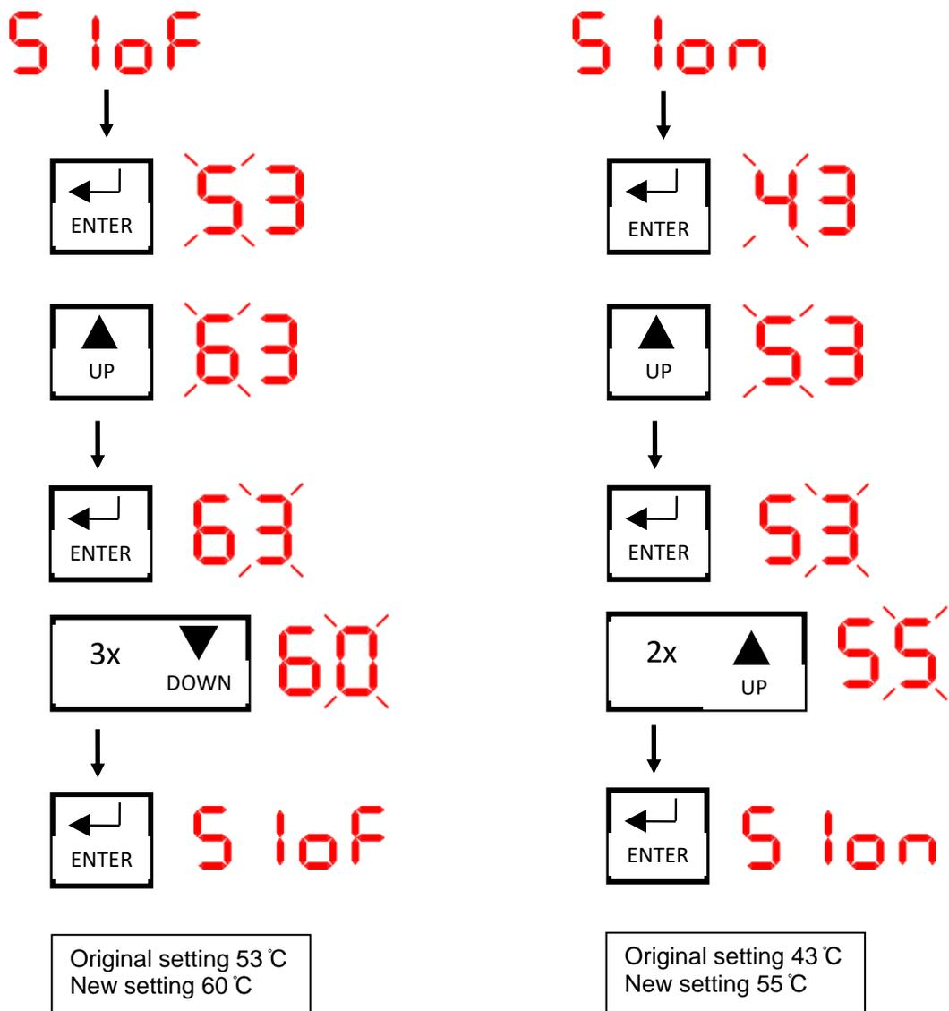
Figure 6.3.2-3 Illustration of the procedure for setting of parameters (temperature)
