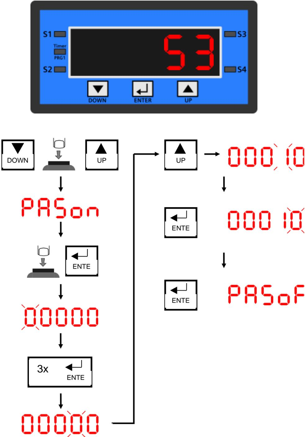
Figure 6.3.2-1 Illustration of the procedure of enabling access to parameters (temperature)
