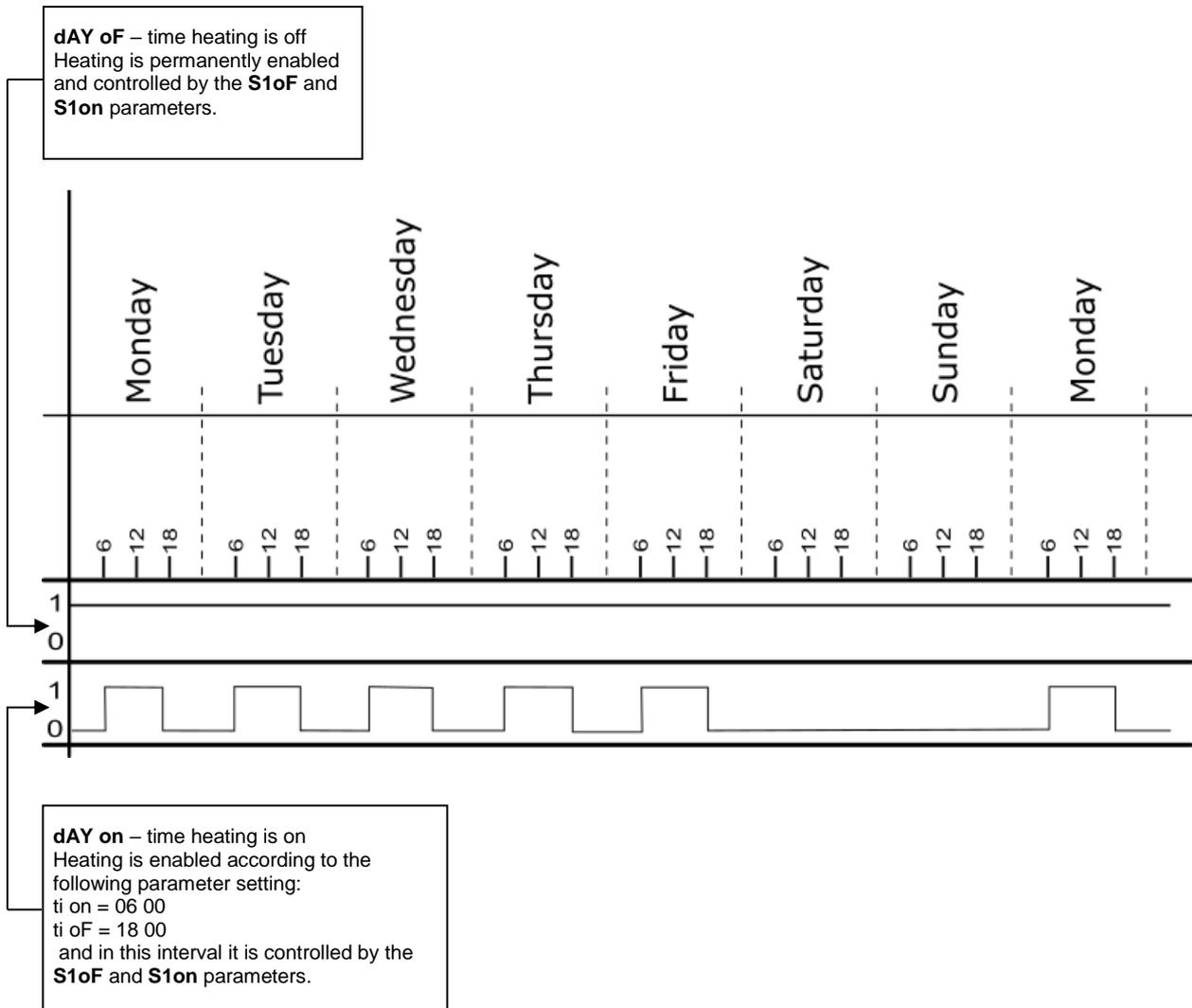
**Figure 6.3.2-6 Diagram of switching the heating element on and off with the activated and deactivated time heating**
