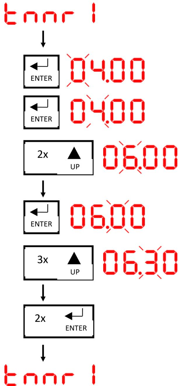
Figure 6.3.2-5 Illustration of the procedure for changing the washing time parameters
