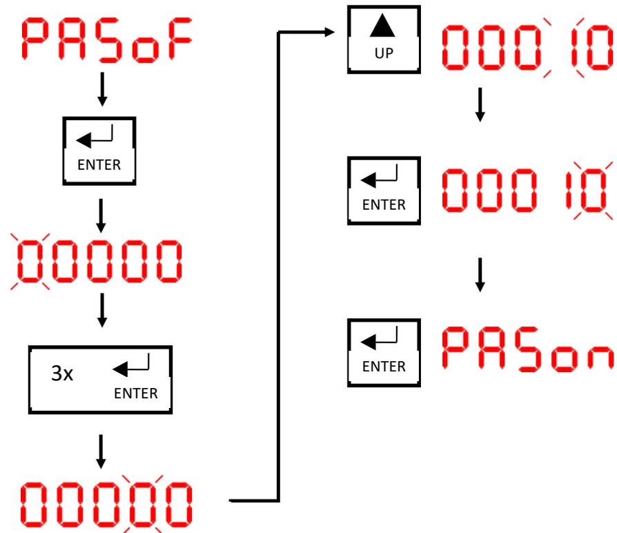
Figure 6.3.2-2 Illustration of the procedure for disabling the access to parameters
