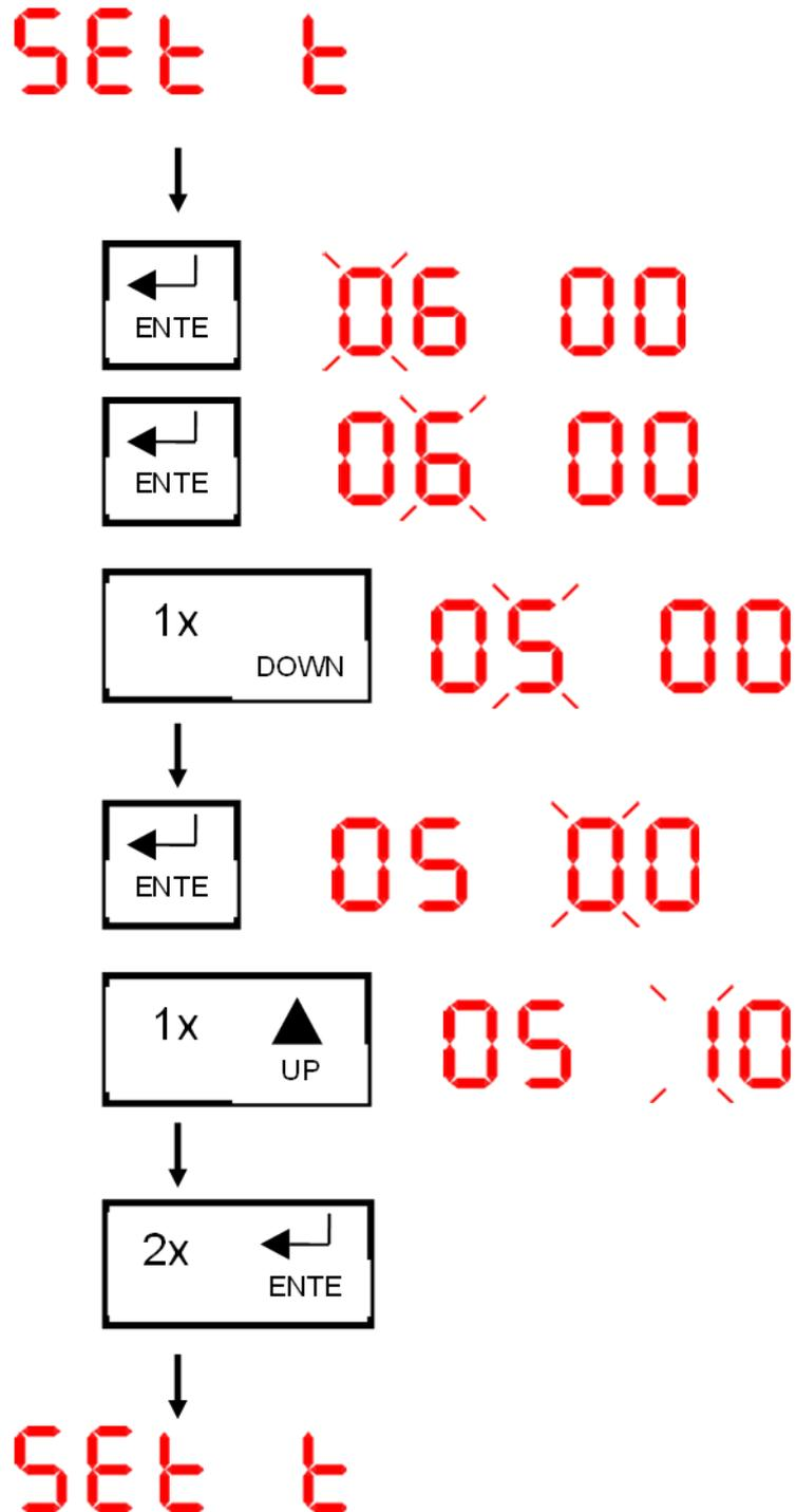
**Figure 6.3.2-9 Illustration of the procedure for entering the date and time**
