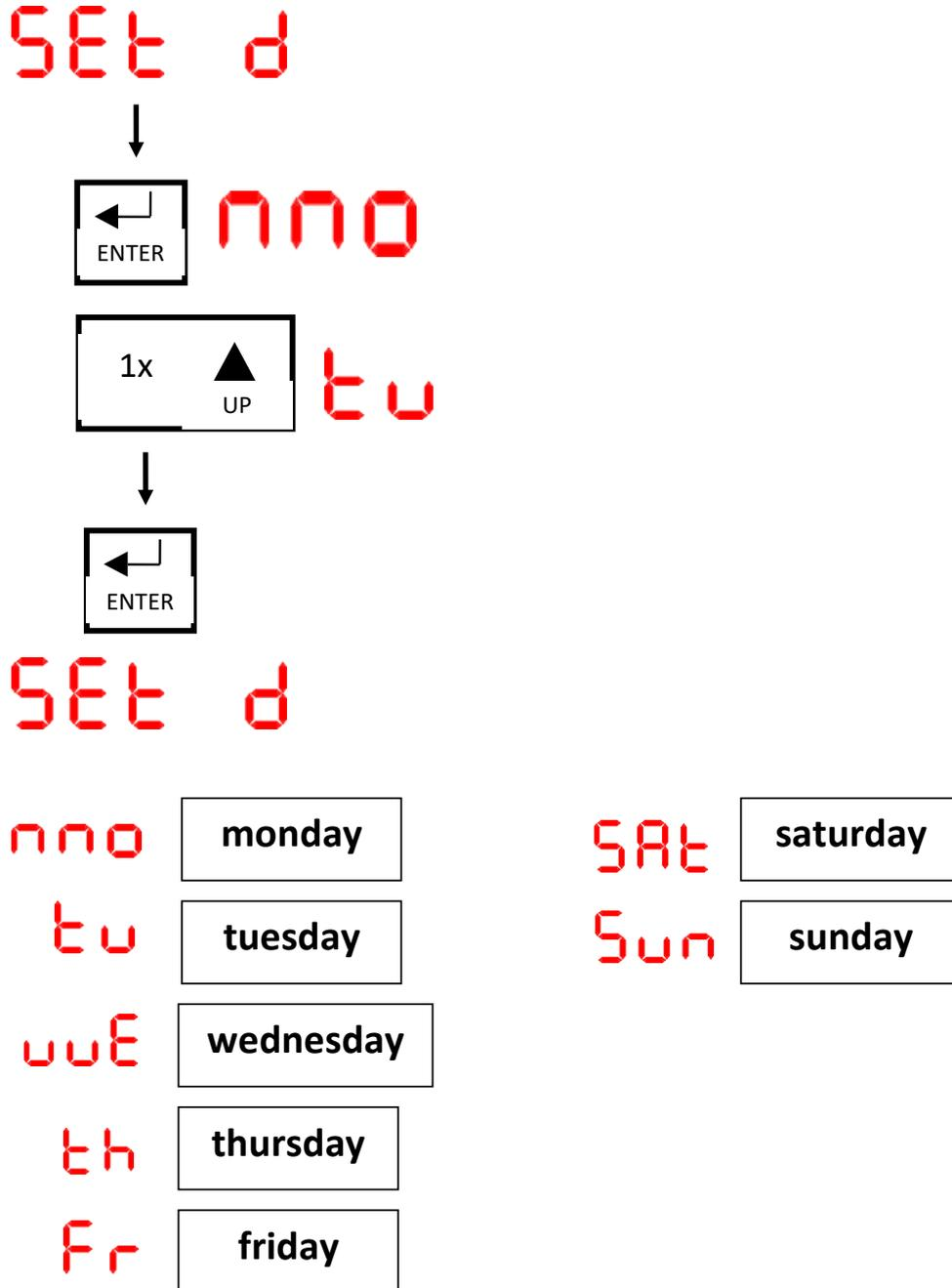
**Figure 6.3.2-8 Illustration of the procedure for entering a day in the week for activation and deactivation of time heating**
