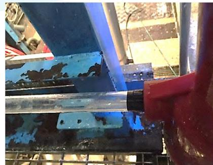
See through tubes, biofilm removed
